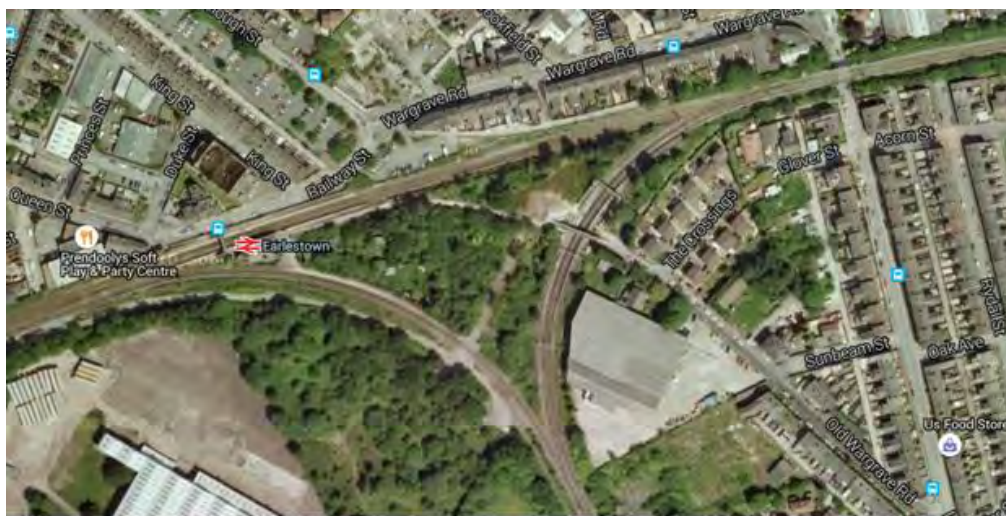
Aerial view of Earlestown Station showing the world's first railway junction or 'wye'
